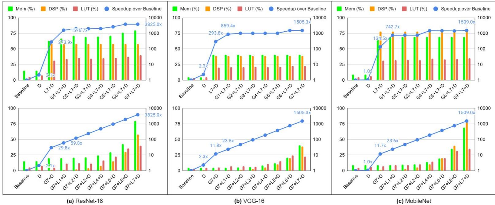
$D$ ,  $L\{n\}$ , and  $G\{n\}$  denote directive, loop, and graph optimizations, respectively. Larger  $n$  indicates larger loop unrolling factor and finer dataflow granularity for loop and graph optimizations, respectively.
